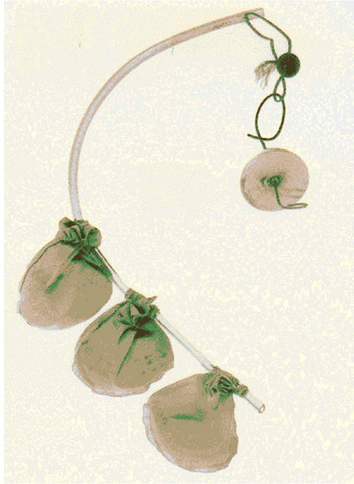
Figure 2. Showing plastic tubing and attachment of nylon bags for suspension in the rumen.
