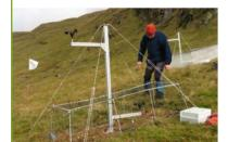
The effectiveness of shelter-netted cages is being measured using anemometers.
