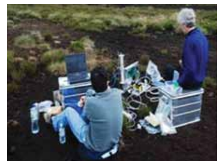
Figure 6 Field application in Scotland of new system for detecting isotopic differences in CO 2 emissions to estimate relative contributions of plant and soil organic matter to C fluxes
