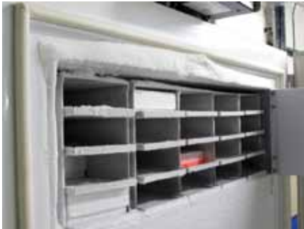
Figure 10 Minus 80°C freezer being used to store soil DNA samples from NSIS-2
