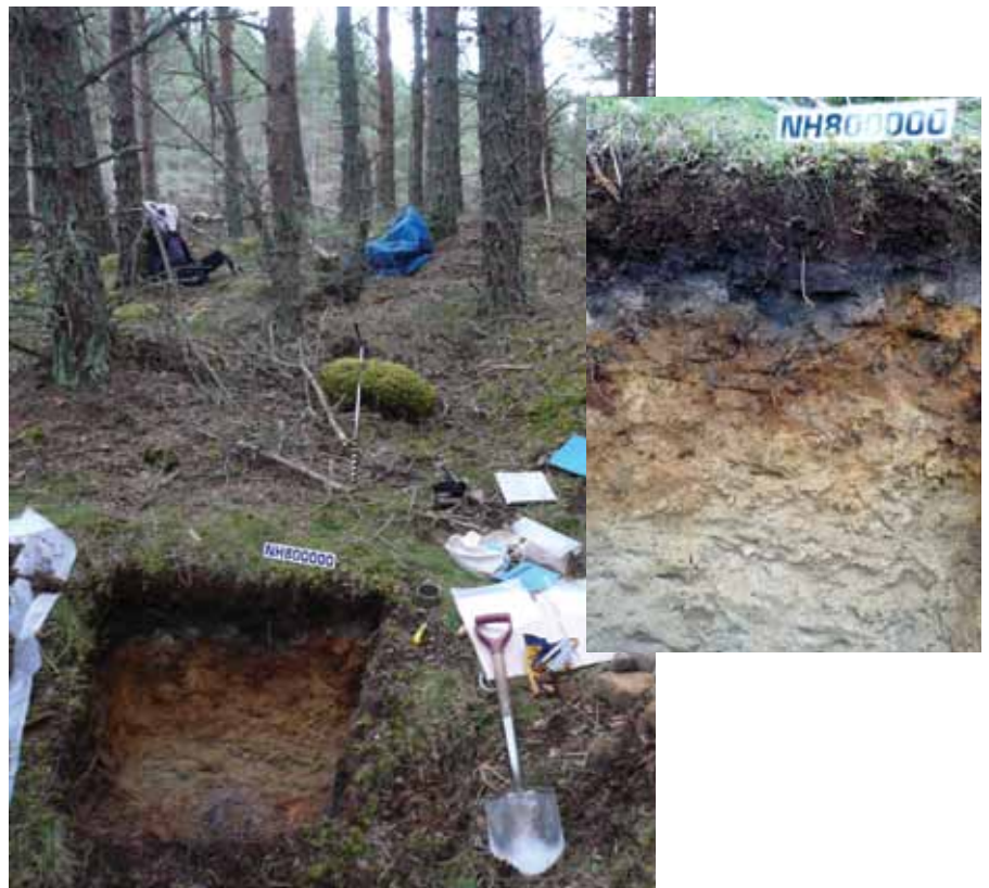
Figure 3 An NSIS-2 resampling site showing the location of the central profile pit. Inset shows a typical podzolic soil under Scots pine showing classical sequence of horizons.
