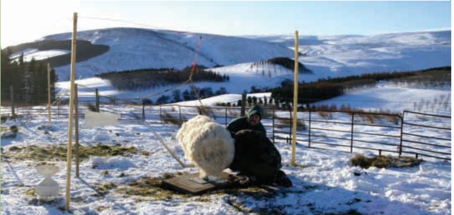
Meteorological station and thermal models of sheep (right) and red deer (back) deployed in the study area.
