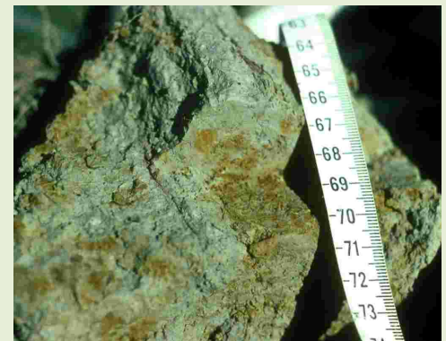
Block of gleyed soil with distinct mottles - grey colours denote gradual depletion of iron because of reducing conditions, "rusty" mottles depict zones enriched with ferric compounds within well-aerated pathways such as old root channels or distinct pores.
