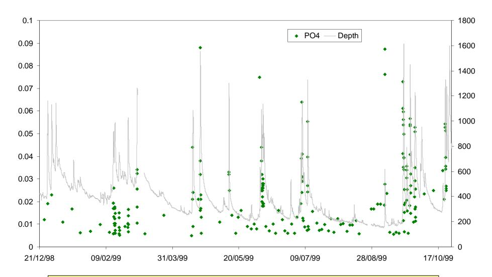
An example of typical information collected at the monitoring station. This example shows the change in flow during 199 and the dots show differences in phosphate in collected samples. Phosphate is associated with sediment particles washed into the stream. When soil is lost and washed off the fields during storms the concentrations of phosphate rise.
